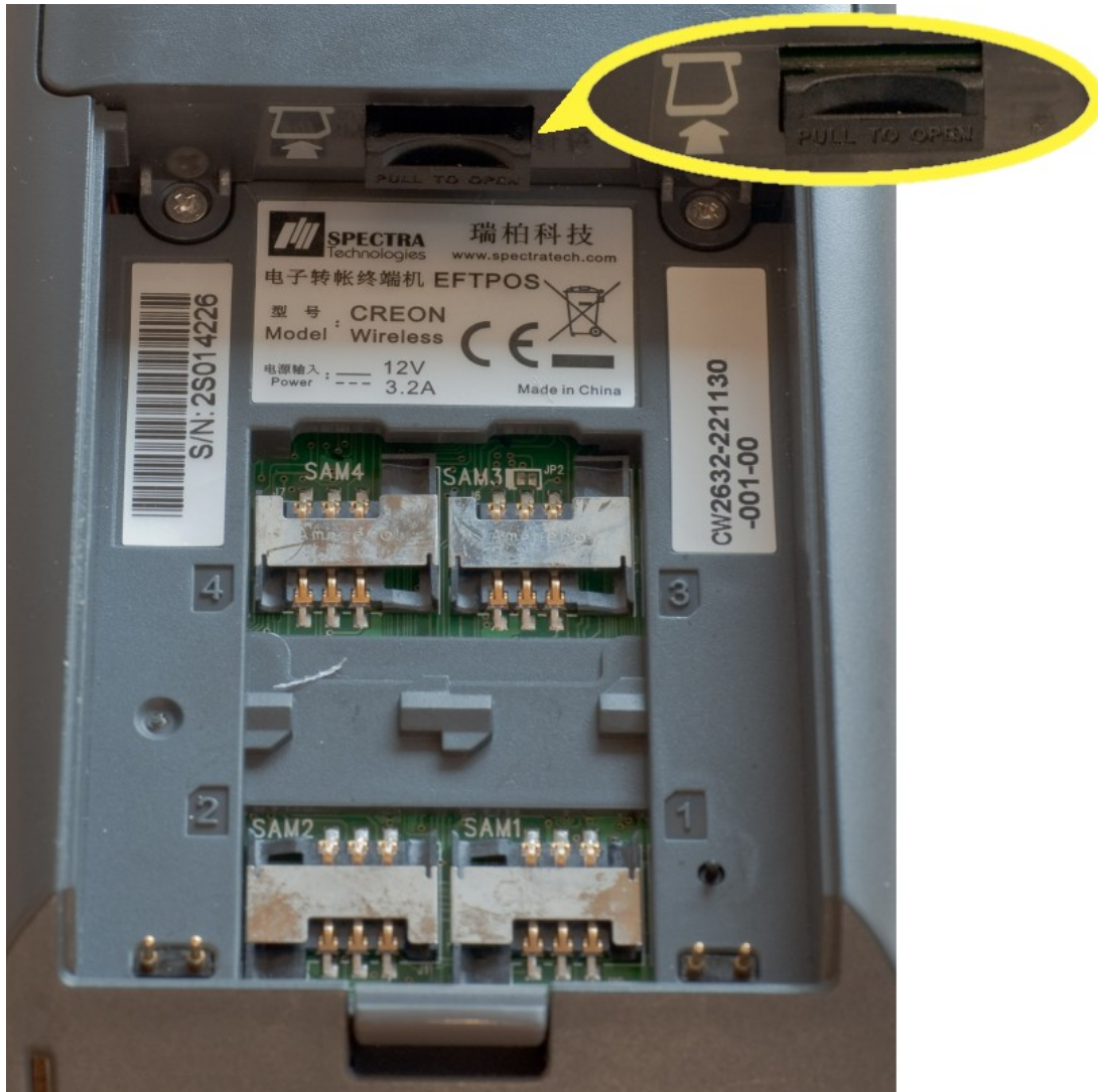
Figure 3: The SIM card must be inserted into the slot (indicated by the circle) as shown by the image next to the SIM slot (also indicated by the circle).
