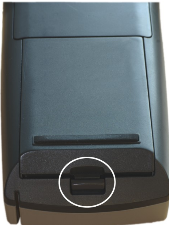
Figure 2: The battery of the Creon terminal can be removed by pressing down on the latch (indicated by the circle).
